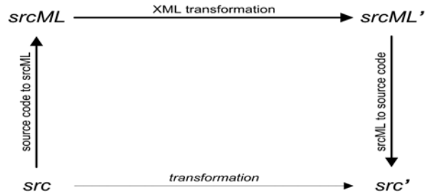
Figure 1. With srcML source-code transformations, such as refactoring, are raised to the level of XML transformations. The source code is translated into equivalent srcML, the srcML undergoes XML transformation, and the resulting srcML is translated back to source code.
